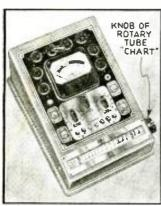
Modern tube checker includes built-in tube listing. (1423)
